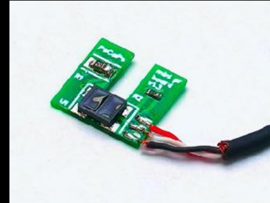
photomicrosensor on encoder board (EE-SY193 by omron [1] )
